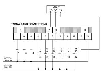
Section 5.4.2 Typical Brush Wear Sensor Connections
